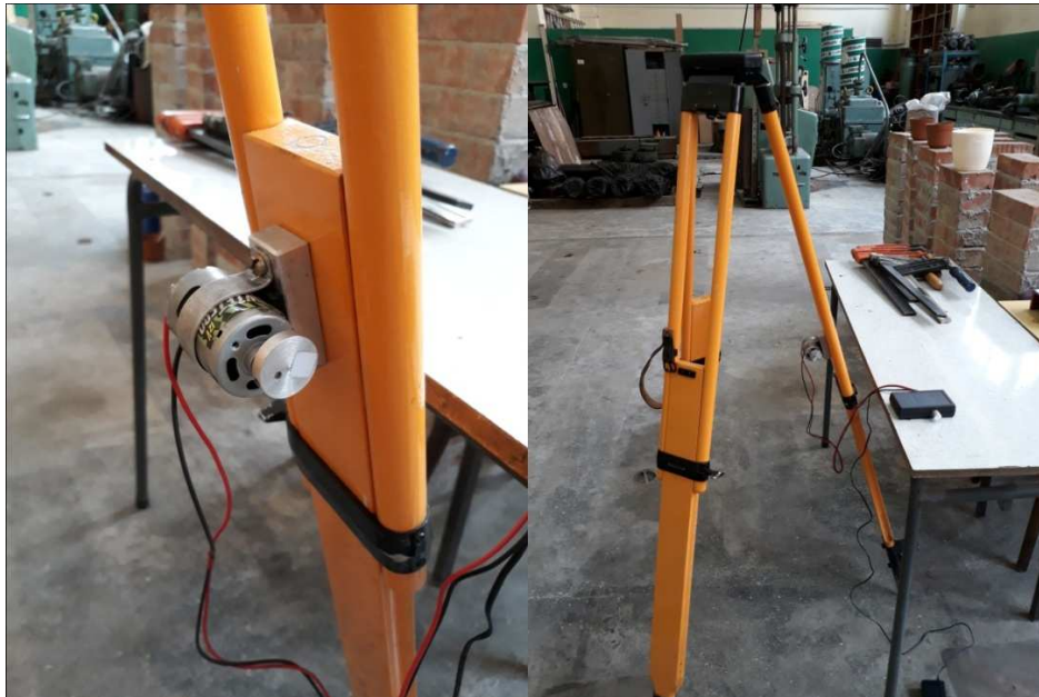
Fig. 1. The tripod with engine generating vibrations
